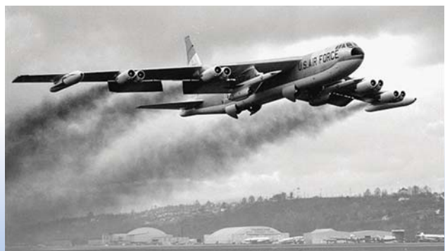
B-52 with Hound Dog missile under each wing, taking off. Source: United States Air Force.
